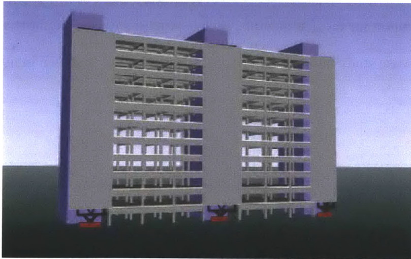
Figure 6.5.1. A model of the case study building (a) as it was before retrofit, (b) with rocking columns installed, (c) with architectural cover
