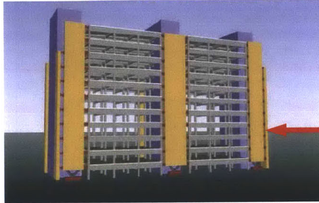
Figure 5.0.1. The case study building model, as retrofitted with rocking walls. The arrow indicates a static shear wall that was damaged during the 2011 earthquake, which was of relatively light intensity in Tokyo.
