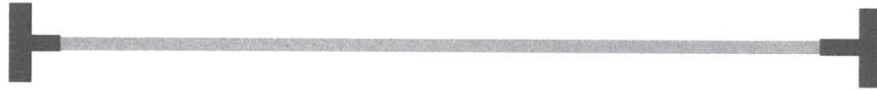
Figure 6.3.2. A schematic plan of a rocking column, using standard structural steel WT shapes, designed for the case study building, to approximate scale, assuming 4 in. members for the truss web.
