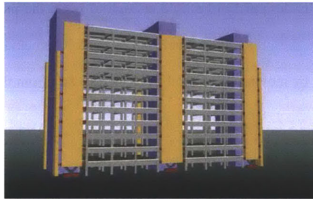
Figure 2.5.1. (a) The case study building in the Suzukakedai Campus of the Tokyo Institute of Technology 27(adapted) , (b) A 3D model of the retrofitted case study building, where yellow represents new structure to be retrofitted 28 .
