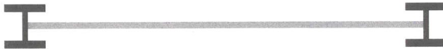
Figure 6.3.1. A schematic plan of a rocking column, using standard structural steel wide flange shapes, designed for the case study building, to approximate scale, assuming 4 in. members for the truss web.
