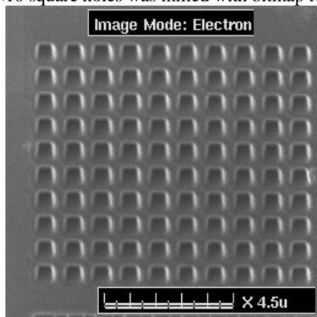
Fig.1 Arrays of square micro-holes on Si (100), each array was milled using rectangular modify box of 10×10 μm<sup>2</sup> with ion dose of 1 nC/μm<sup>2</sup>; 10×10 square holes.
