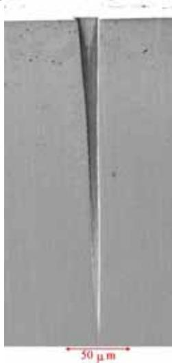
Fig.8 Micro-hole milled on Ni-Be by the FIB with ion dose, ion energy, and beam current of  $160 \text{ nC/mm}^2$ ,  $50 \text{ keV}$ , and  $19 \text{ nA}$ , respectively. Total milling time is  $98 \text{ min}$ . Milling depth is  $246 \mu\text{m}$ .
