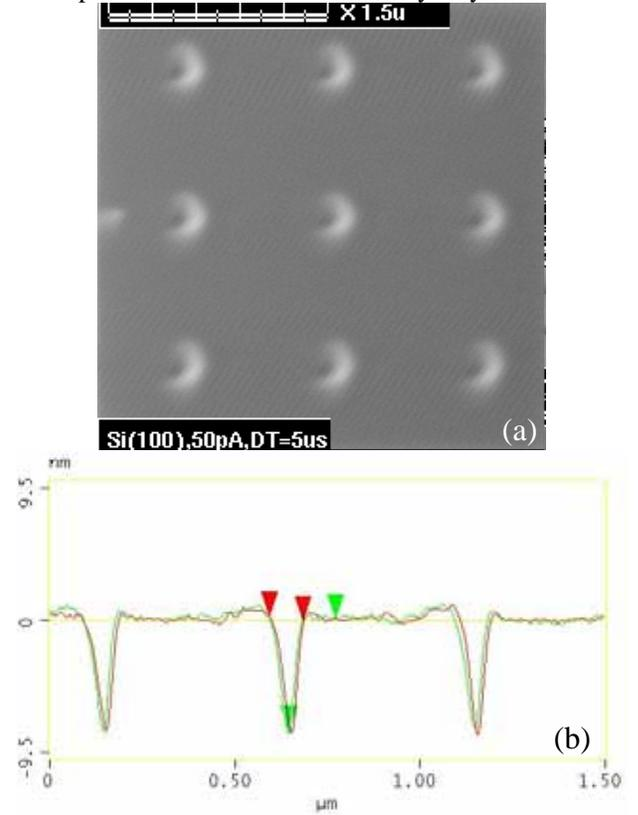
Fig.6 FIB micrograph of a nano-hole array on Si(100) with the pixel space mode but controlled only one scan time for a frame, beam spot size of  $\sim 10 \text{ nm}$ , beam current of 7pA, dwell time of 50 ms. Total scanning time of one frame is 64s. (a) Micrograph of SEM with field emission; (b) two-dimensional profile measured by AFM with tapping mode.
