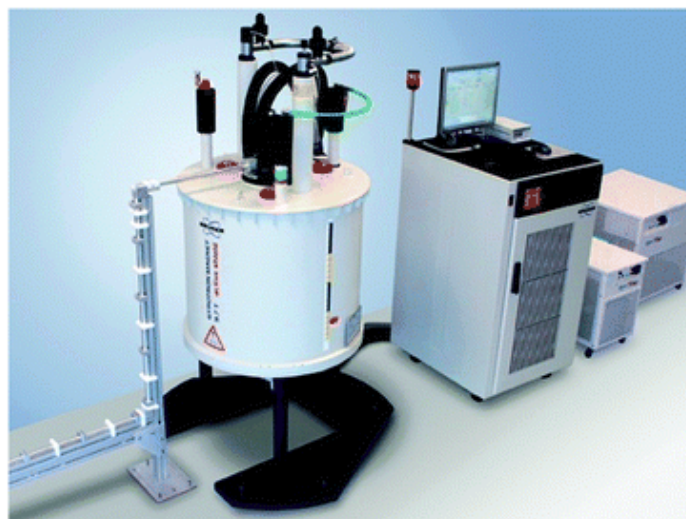
Fig. 11: Commercial DNP/NMR spectrometer with the gyrotron and magnet shown at the left and the control and cooling systems for the gyrotron shown on the right. (Adapted from [16])
