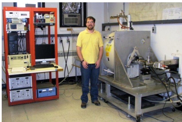
Fig. 9. 140 GHz Gyrotron Oscillator (right), control system (left), grad student Mr. Andrew Casey.
