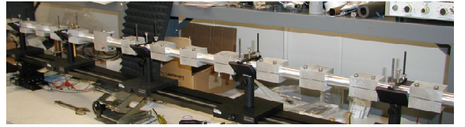
Fig. 20. Photo of the corrugated 22 mm waveguide transmission line of Fig. 18.
