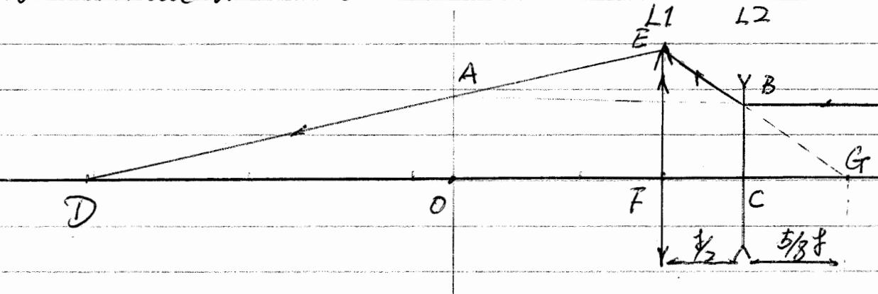
The parallel rays from left will have a virtual focal point at G after passing through Lens L<sub>2</sub>.
