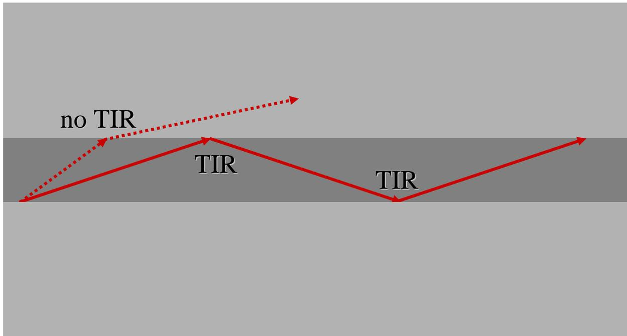
“planar” waveguide: high-index dielectric material sandwiched between lower-index dielectrics
