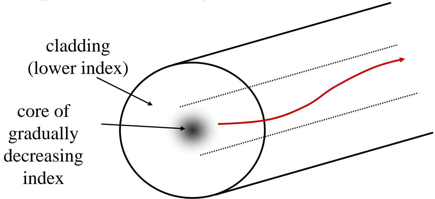
optical rays “swirl” around the axis of the core!
