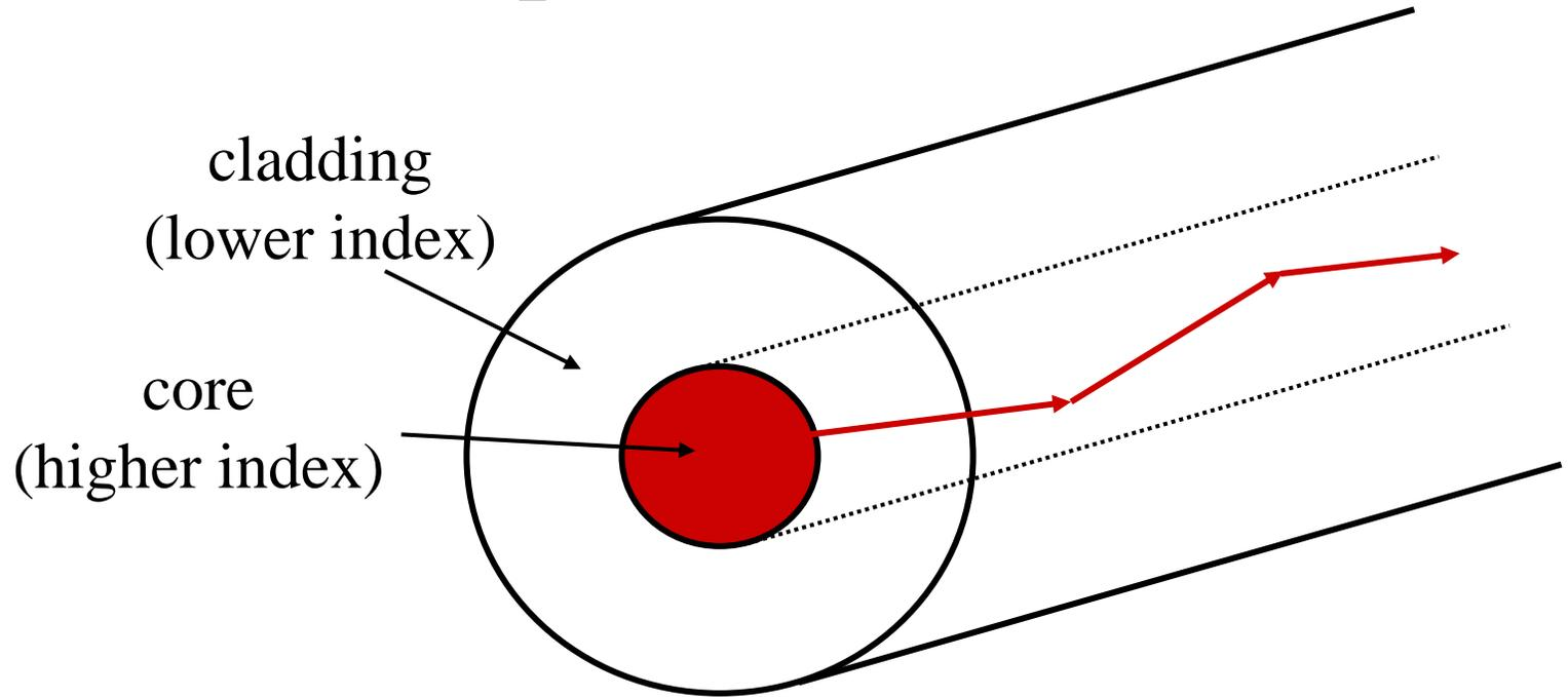
Core diameter = 8-10 $\mu\text{m}$  (commercial grade)
