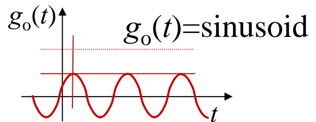
$$g_i(t) = a_0 \cos(\omega_0 t) \Rightarrow g_o(t) = a_0 |H(\omega_0)| \cos(\omega_0 t - \phi(\omega_0))$$
