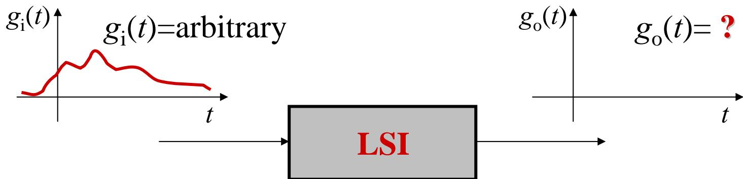
$$g_i(t) = \int g_i(t_0) \delta(t - t_0) dt_0 \quad \xrightarrow{\text{red arrow}} \quad g_o(t) = \int g_i(t_0) h(t - t_0) dt_0$$
