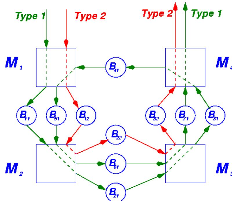
Semiconductor fabrication is highly reentrant.
