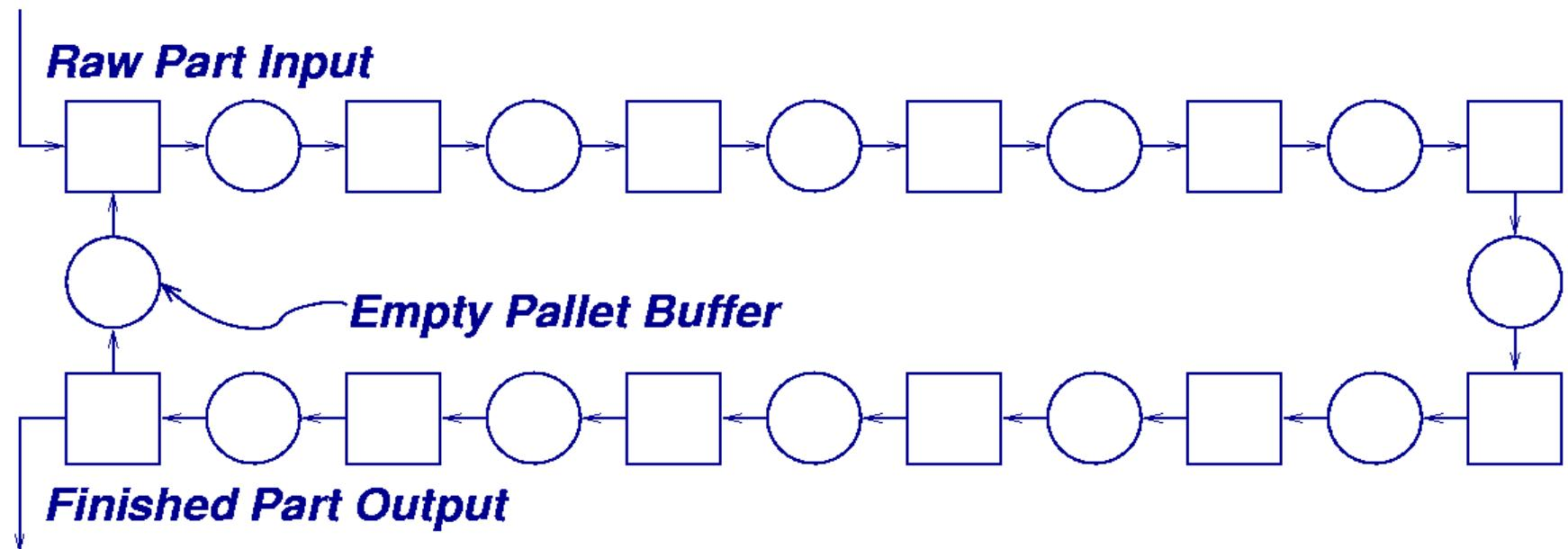
Pallets or fixtures travel in a closed loop.
