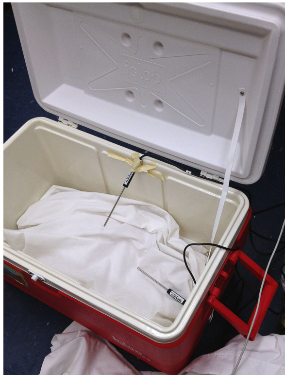
Figure 2.7: A photograph of the Test 2 set-up. A sensor measuring wax temperature enters through the side of the cooler (to the right in this photo).
