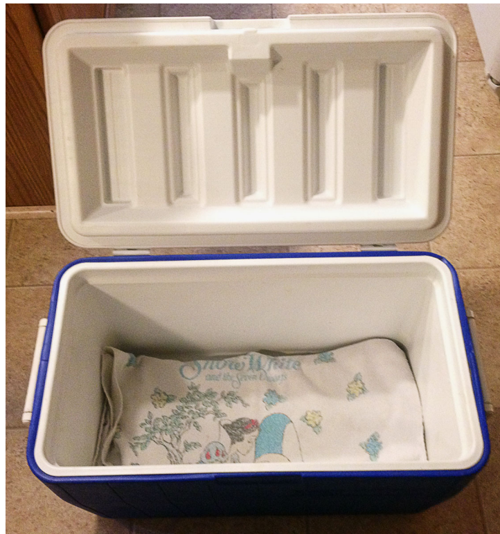
Figure 2.6: Two boxes were placed in the cooler to elevate the sample and provide more insulation underneath. The two bags of wax were placed with one layer of towel above the wax.
