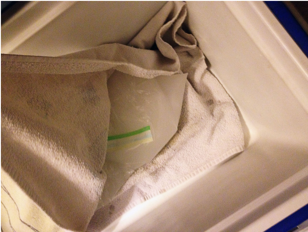
Figure 2.4: The wax, enclosed in a plastic bag for boiling purposes, was placed on top of phone books to accurately represent the height of the chamber. A towel was placed atop the wax to simulate cotton padding or other materials used to cushion the infant.
