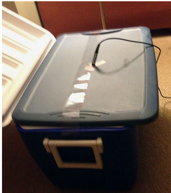
Figure 2.5: Test 1 set-up. A thin plastic lid with a 4.25” TMP probe placed through a small, drilled hole and allowed to hang in the air chamber.
