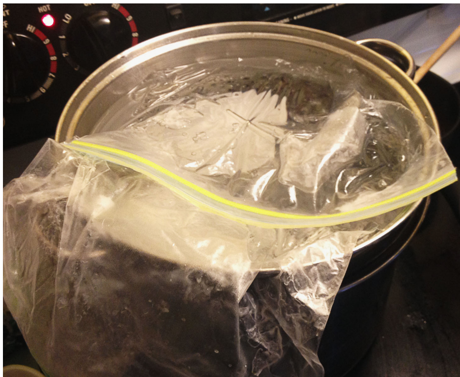
Figure 2.3: Solid wax was placed into gallon-size, zip-top bags and placed into a pot with a straining pot inside. The plastic of the zip-top bags melt easily upon contact with metal surfaces directly touching the burner, so the second pot is a necessity (see Figure 2.2 for an illustration).
