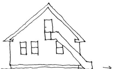
STAIR MOVED FORWARD TO REGAIN USE OF WINDOW; PRIVACY RETAINED FOR ALL THREE WINDOWS
