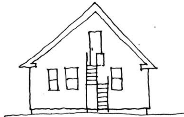
SCISSOR STAIR DOES NOT BLOCK WINDOWS BUT MAY BE MORE VISIBLE FROM THE STREET.
