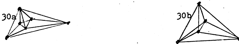
Figure 30. Simply-representable graphs. Both of the figures shown above are not simply-representable in two dimensions.
