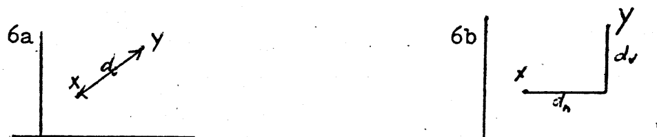
Figure 6. Metrics on E^2 . The natural Euclidean metric is shown in 6a. d(x,y) = d_0 . The metric d(x,y) = d_h + d_v , is shown in 6b.
