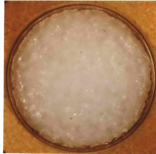
Figure 3.3 Saturated Liquid Nitrogen (b. pt. -196\text{ C} ) Film Boiling on a Water Surface Vessel Diameter Was 14.5 cms and the Water Was at 24\text{ C} at t=0
