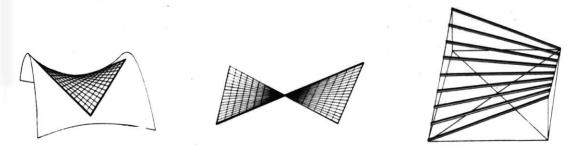
Hyperbolic paraboloid is warped double-curved surface, saddle shaped, generated by straight line that slides along two straight line directrices not in same plane and remains parallel to plane director.
