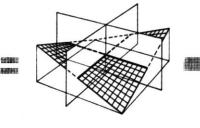
Although it is double-curved surface, its intersection with vertical plane parallel to edges of surface produces straight lines. Only central lines are horizontal.
