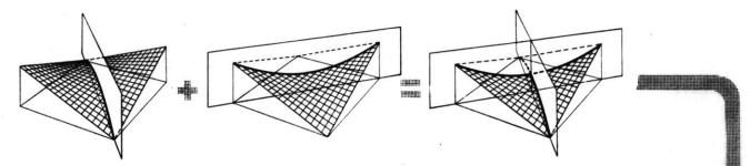
Any intersection of surface with vertical plane parallel to its diagonals produces parabolic curves
