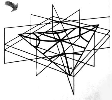
Synthesis of sections between surface and horizontal and vertical planes.
