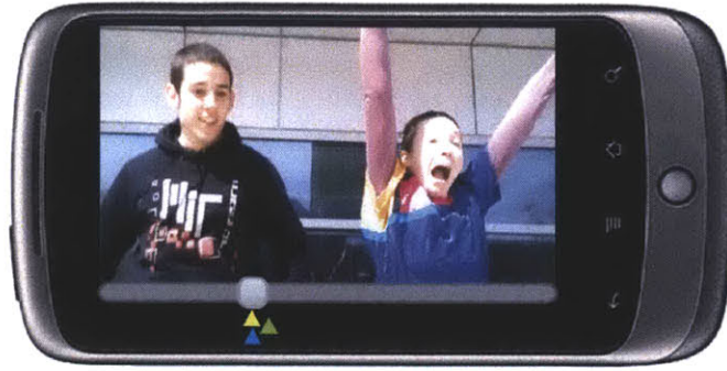
Figure 1-3: Adrenaline’s realtime crowds operate a camera shutter by choosing the most photographic moment seconds after it happens. Crowd members’ current votes on the best frame appear as colored triangles below the timeline.
