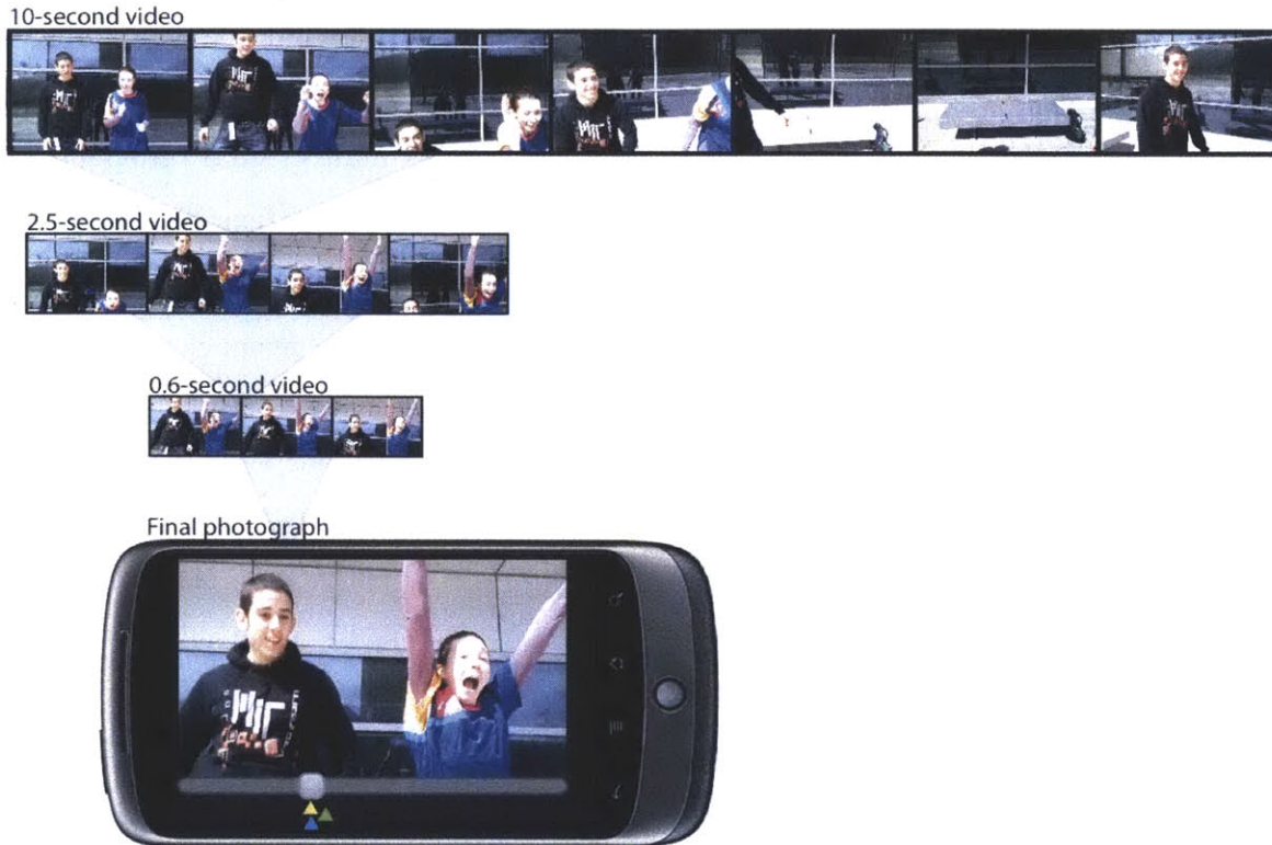
Figure 5-1: Adrenaline is a camera that uses crowds to find the right moment for a picture by capturing ten-second movies. It looks for early agreement to filter the timeline down quickly to a single frame. A photo is typically ready about one second after the user reviews the movie.
