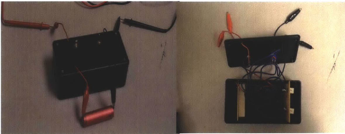
Figure 4: Battery Discharge Box
