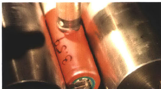
Figure 13: Crush Test of the 18650 Cell by a Hemispherical Punch
