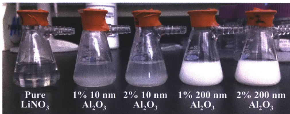
Figure 22. LiNO 3 solutions with (from left to right) pure LiNO 3 , 1% Al 2 O 3 (10 nm), 2% Al 2 O 3 (10 nm), 1% Al 2 O 3 (200 nm), and 2% Al 2 O 3 (200 nm).
