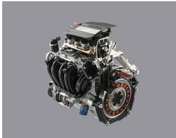
Figure 16: Honda 3-Stage i-VTEC + IMA system, as used in the Civic Hybrid 2005.
