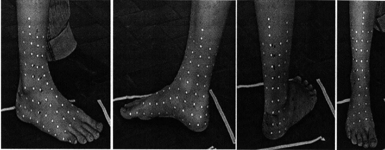
Figure 2.3: Sample images from Marreiros's study of the human ankle joint. Note the 2cm grid of infrared markers placed on the body [11].
