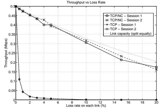
Fig. 13. Throughput vs loss rate for TCP and TCP/NC
