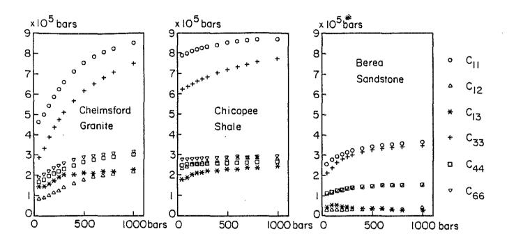
FIG. 7. Stiffness constants vs. confining pressure.  $C_{ij}$  constants are defined by equations (1) to (5).
