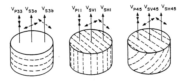
FIG. 2. Velocities measured in this experiment. Solid arrows represent directions of wave propagation; dashed arrows represent directions of particle motion, dashed lines in the sample indicate bedding planes in Berea Sandstone and Chicopee Shale and rift planes in Chelmsford Granite.
