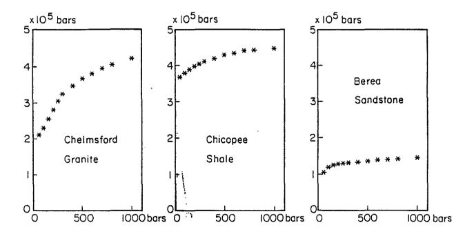
FIG. 10. Dynamic bulk modulus vs. confining pressure.
