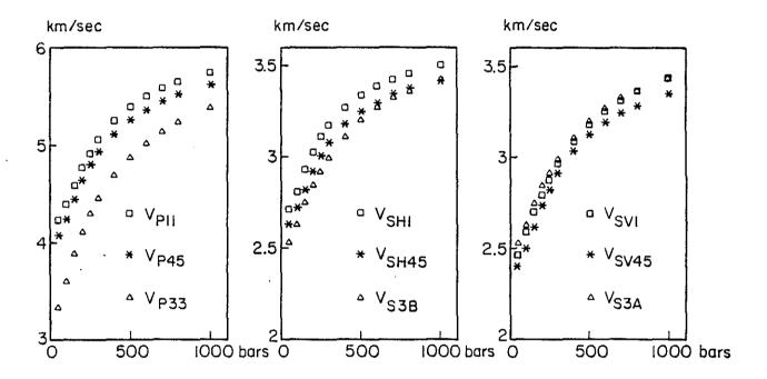
FIG. 4. P-, SH-, and SV-wave velocities in different directions for Chelmsford Granite. Subscripts indicating directions are defined in Fig. 2.
