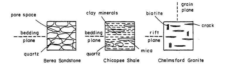
FIG. 11. Schematic diagrams showing the petrofabric characters of rock samples used in this experiment. In Berea Sandstone, most of the long axes of the quartz grains are parallel to the bedding plane. In Chicopee Shale, most of the cleavage planes of mica and the long axes of other constituent minerals are parallel to the bedding plane. In Chelmsford Granite, most of the penny-shaped cracks are parallel to the rift plane and most of the biotite cleavage planes are parallel to the grain plane.
