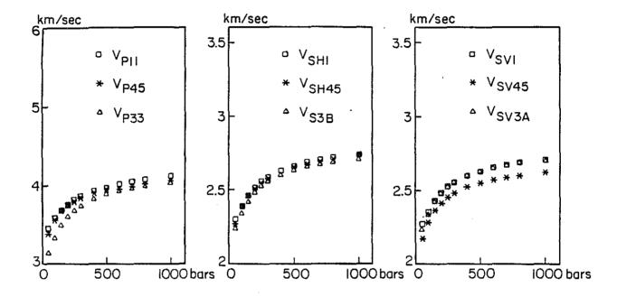
FIG. 6. P-, SH-, and SV-wave velocities in different directions for Berea Sandstone. Subscripts indicating directions are defined in Fig. 2.
