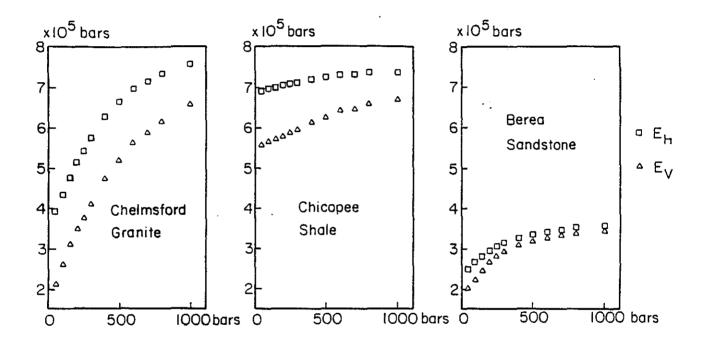
Fig. 8. Dynamic Young's moduli vs. confining pressure.  $E_v$  = Dynamic Young's modulus perpendicular to the plane of isotropy.  $E_h$  = Dynamic Young's modulus parallel to the plane of isotropy.
