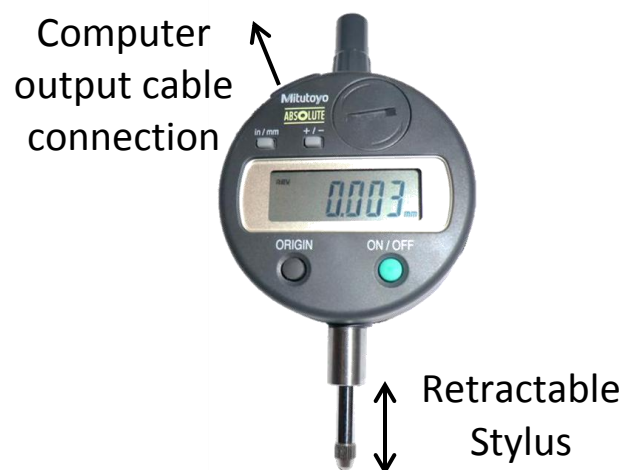
Figure 3.8: Digital Indicator. The Mitutoyo ID-S112TB digital indicator is used in the apparatus to measure shaft displacement during stiffness testing. The stylus is placed in contact with the spindle and retracts or extends to measure displacement.
