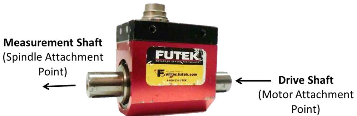
Figure 3.15: FUTEK Rotary Torque Sensor. A FUTEK FSH02057 rotary torque sensor will be used in the apparatus to measure running torque. The sensor must be axially aligned with and physically connected to a motor and the spindle in order to measure effectively.
