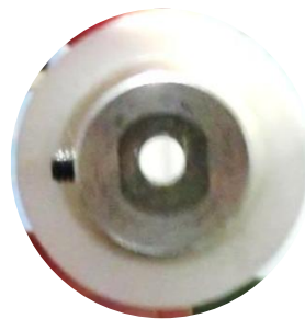
Figure 5.8: Spindle pulley. A vee-clamp was used to hold the pulley in place as the non-circular pocket shown was milled.
