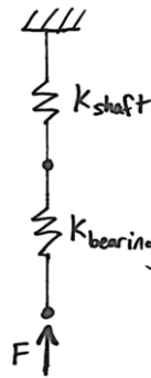
Figure A.3: Superposition of stiffness contributions. The bearing stiffness and shaft stiffness can be superimposed to find the overall spindle stiffness.
