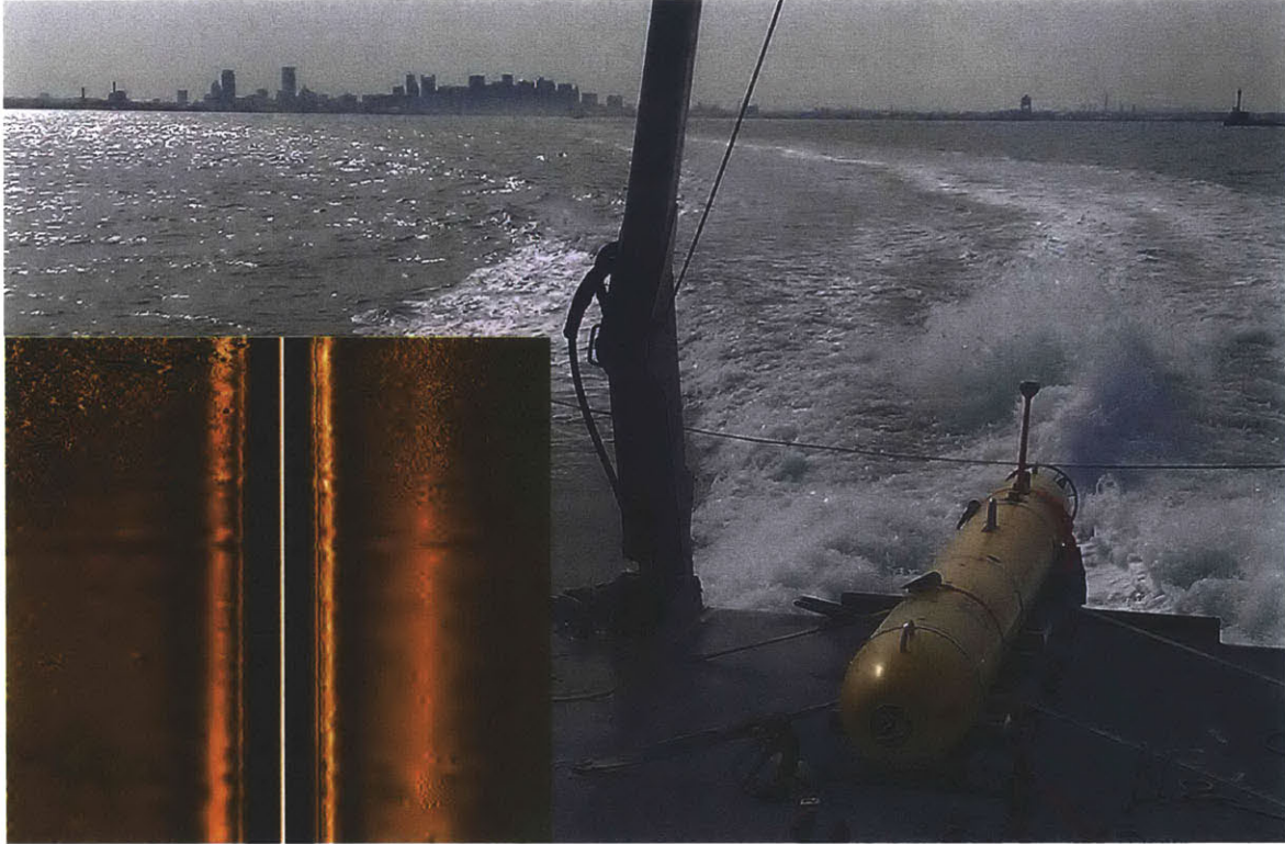
Figure 5-3: Bluefin 9 AUV prior to deployment, and the sonar imagery transmitted during the dive.
