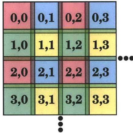
Figure 3-15: A schematic of the grid used for subsampling the classification mask, illustrating the overlap between adjacent cells. Note that the lack of overlap at image edges means that a simple interpolation would bias the resulting mask.
