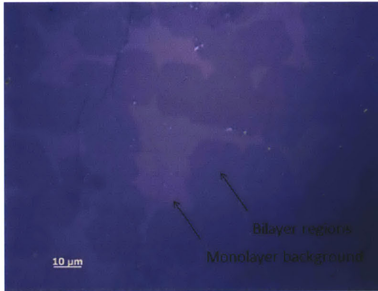
Figure 4. Typical optical images of graphene films on Si wafer with 300 nm thick SiO 2 .
