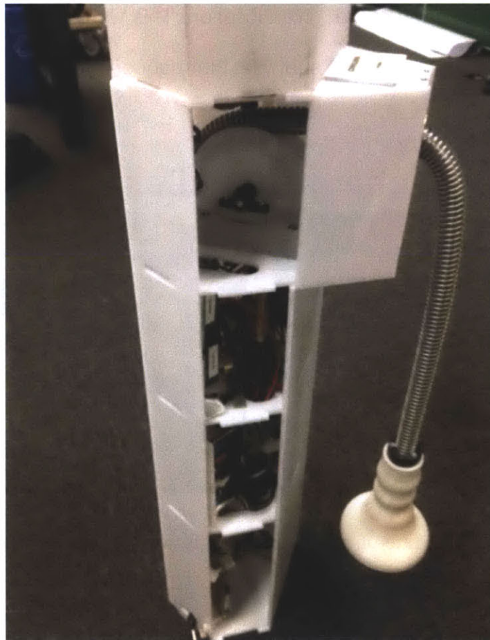
Figure 20: Internal electrical system and pulley for retractable arm
