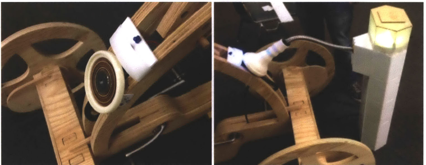
Figure 18: Female connector (left) and inserted male charger (right) with locking mechanism activated
