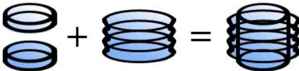
Figure 3.4: Two geometric sections comprise the entire bellows volume.
