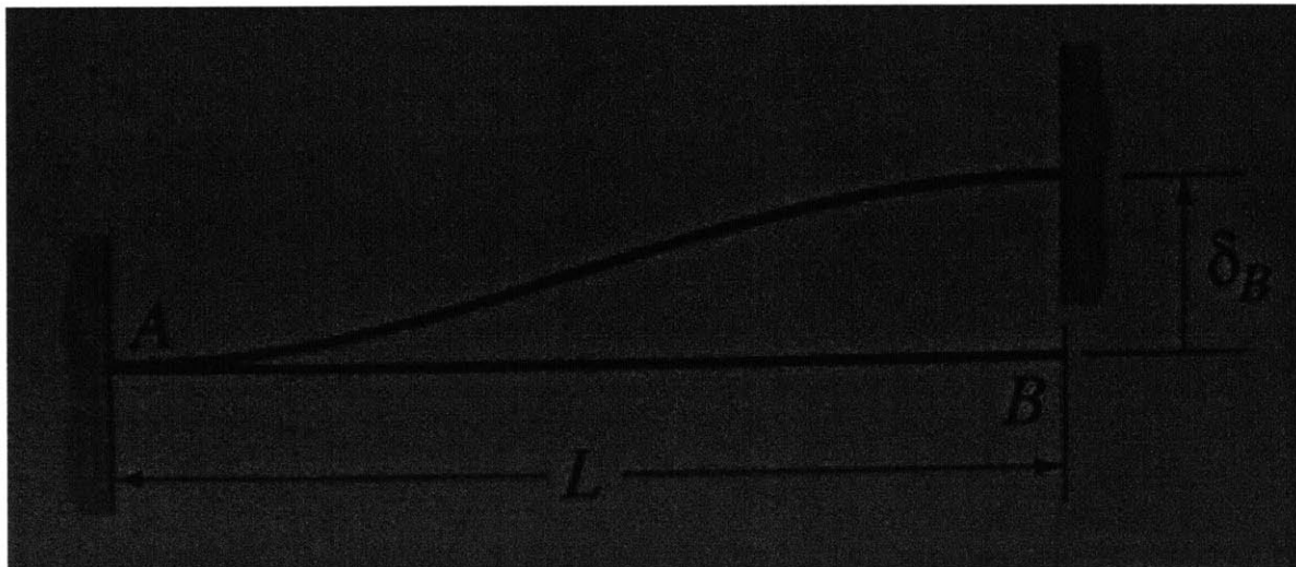
Figure 4-6: A profile view of the flexure found in the photodiode stand flexures, the highest moment of which can be found at point B, where there is a deflection of \delta_B . [10]
