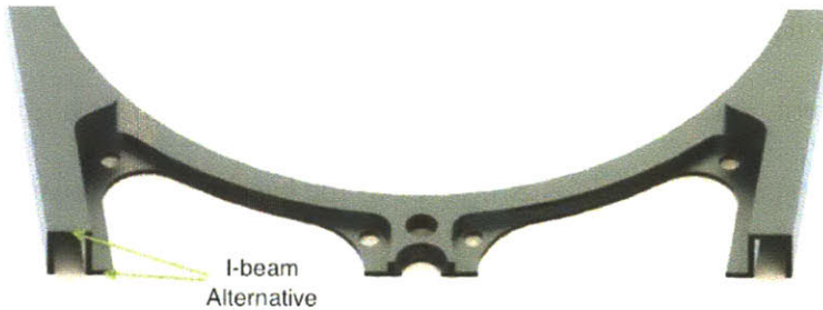
Figure 3-4. Cross section of Frame. Showing the design used in order to approximate an I beam in designing the claw's frame
