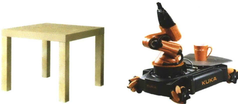
Figure 1-1 The components of the class challenge. On the left is the table, with four legs that had an approximately two inch square cross section. This was the item that needed to be attached by the robot. The robot is a miniature educational version of the German industrial robotics company Kuka's mobile robotic arm. [3]
