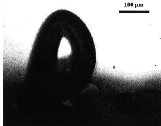
Figure 4.2.6. An unusually-shaped bubble that may be trapped in a small hydrophobic area within a hydrophilic region. This surface feature produces a tall, thin bubble that has a small contact area with the surface.
