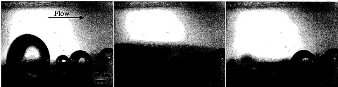
Figure 3.4.1. An example of a series of video frames which indicate that the departure of a bubble was premature and thus should not be used in data analysis. In this case the bubble appears to have been pushed off by another bubble, as indicated by the shadow in the central image.
