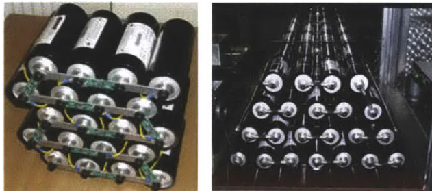
Figure 3-3: Interconnection of commercial, discrete ultracapacitors to form banks in order to minimize voltage variation and/or maximize energy utilization.
