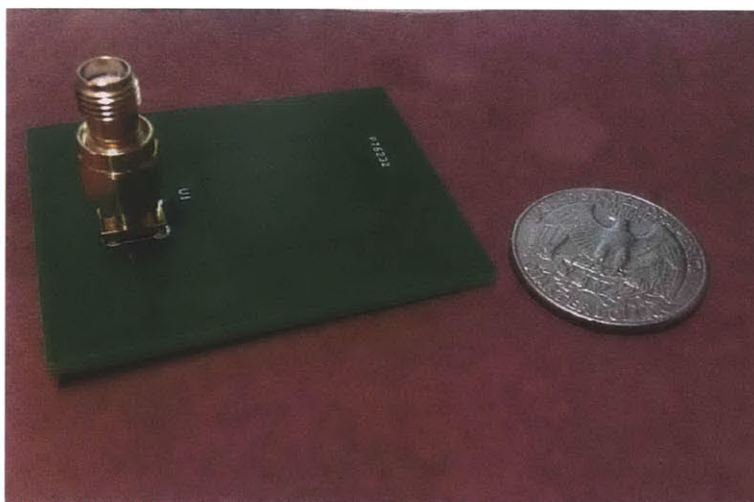
Figure A-4: Simple PCB loop antenna used for benchmarking.
