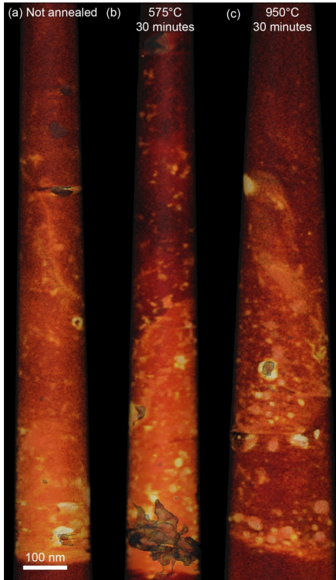
Figure 6.15. HAADF-STEM Tomography reconstruction of selenium-hyperdoped silicon extracted from the center of the polycrystalline peaks, showing selenium distribution (a) before annealing (b) after a 30 minute anneal at 575°C, and (c) after a 30 minute anneal at 950°C.
