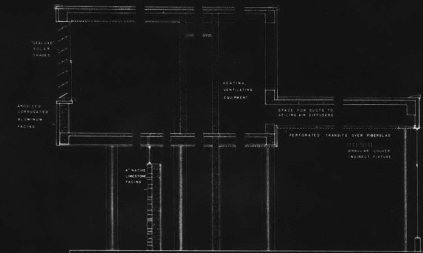
STRUCTURAL DETAILS AT TYPICAL SECTIONS - SCALE 1/16" = 1'-0"
