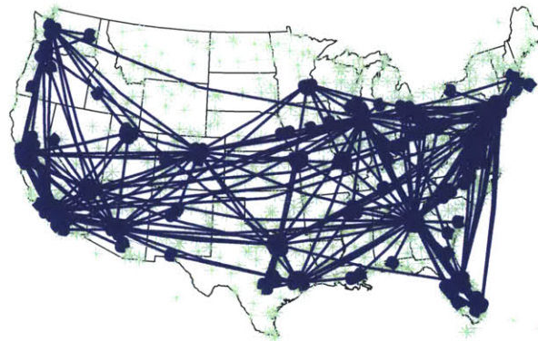
Figure 2-4: Simplified NAS network showing links with at least 10 flights a day. The light green icons denote airports in the original dataset that are not included in the simplified network.
