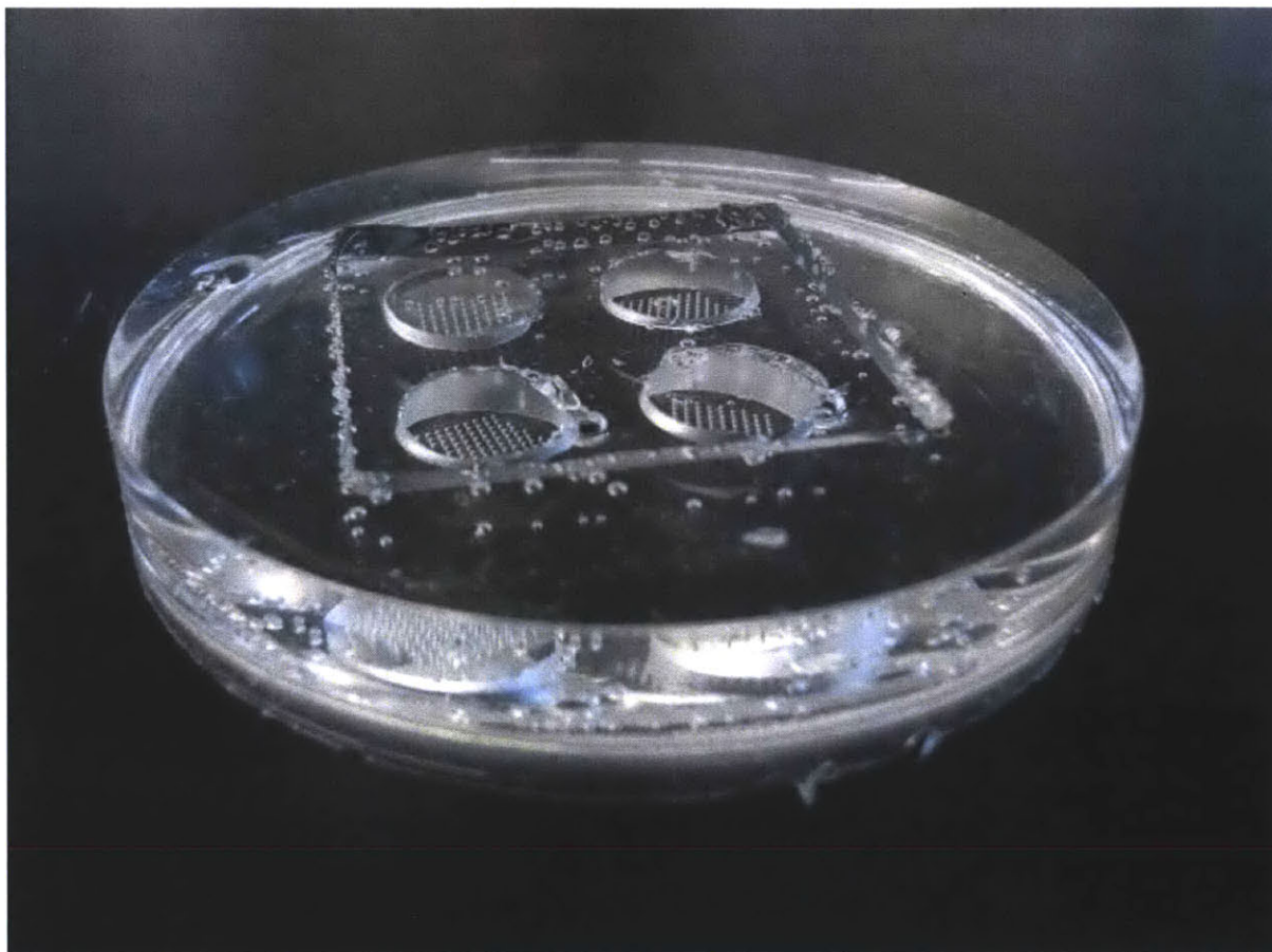
Figure 8: PDMS mold used to synthesize microneedles
