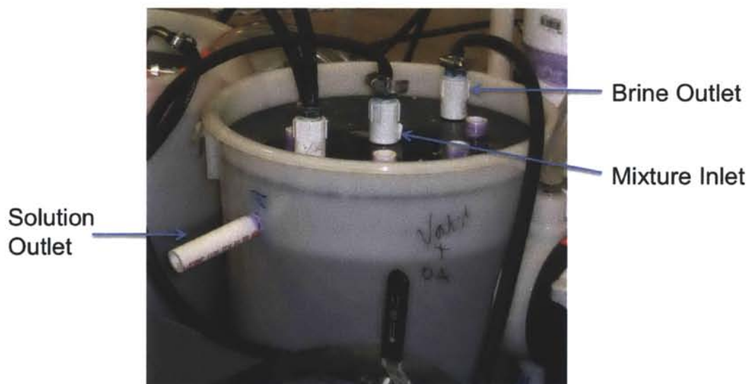
Figure 3-7: The final design of the gravitational separator with the insert from Figure 7 inside the five-gallon bucket, and the outlet pipe extending out from the top. The mixture from the mixer enters the gravitational separator through flexible tubing, brine is extracted to a waste bucket below the gravitational separator, and the desired solution flows through the outlet pipe and into the chiller without the use of any pumps or input energy.
