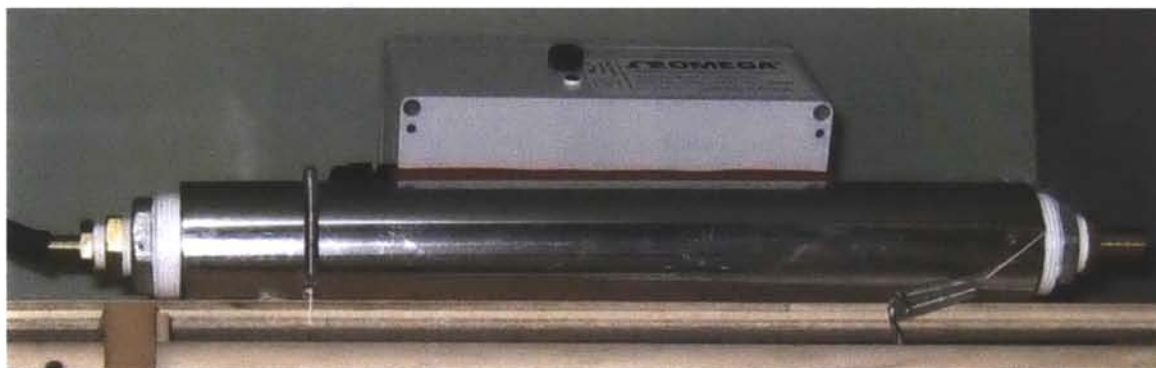
Figure 3-2: Liquid flow-through heater used to heat the solvent or the contaminated water before entering the mixer.
