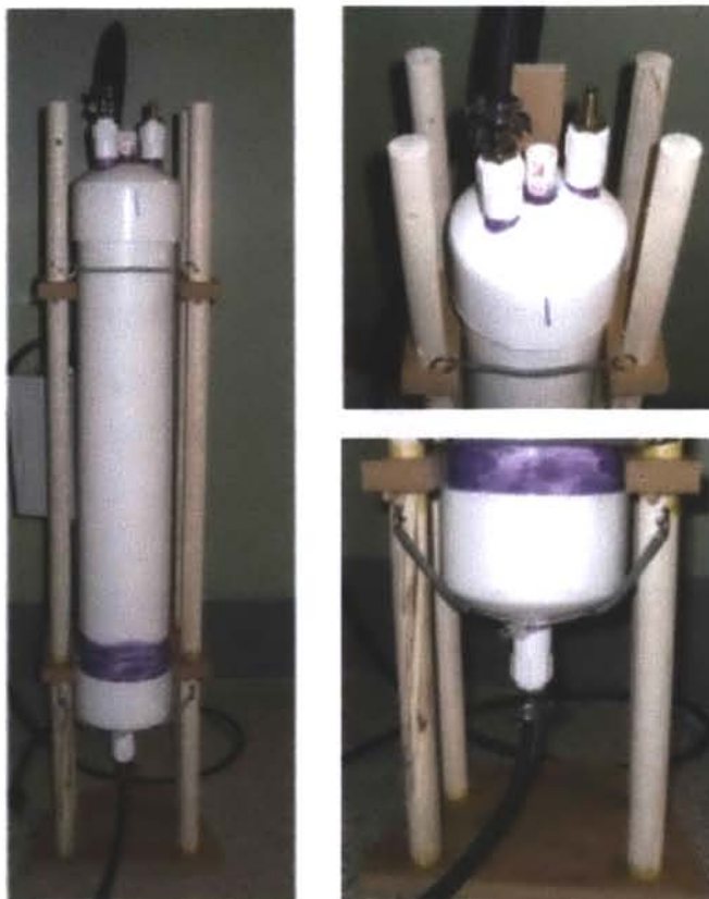
Figure 3-3: First iteration of the containment vessel and stand with close up views of the top and bottom caps. The top cap has two ports for the solvent and contaminated water and a hole in the middle for the stirrer rod. The bottom has one port for the output of the mixture to the gravitational separator. The stand uses springs to remove vibrations and allow the PVC piping to expand and contract.
