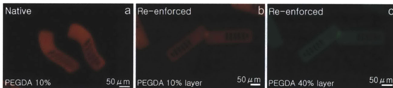
Figure 5.11: Reinforced barcoded particles (a) Fluorescent image of soft PEG particles that were bent due to the mechanical instability. (b-c) Fluorescent images of reinforced barcoded particles. The sandwiched particles consisted of three layers: (1) two soft porous layers in the top and bottom of the particles (Red) and (2) a hard supporting layer in the middle of the particles (Green).
