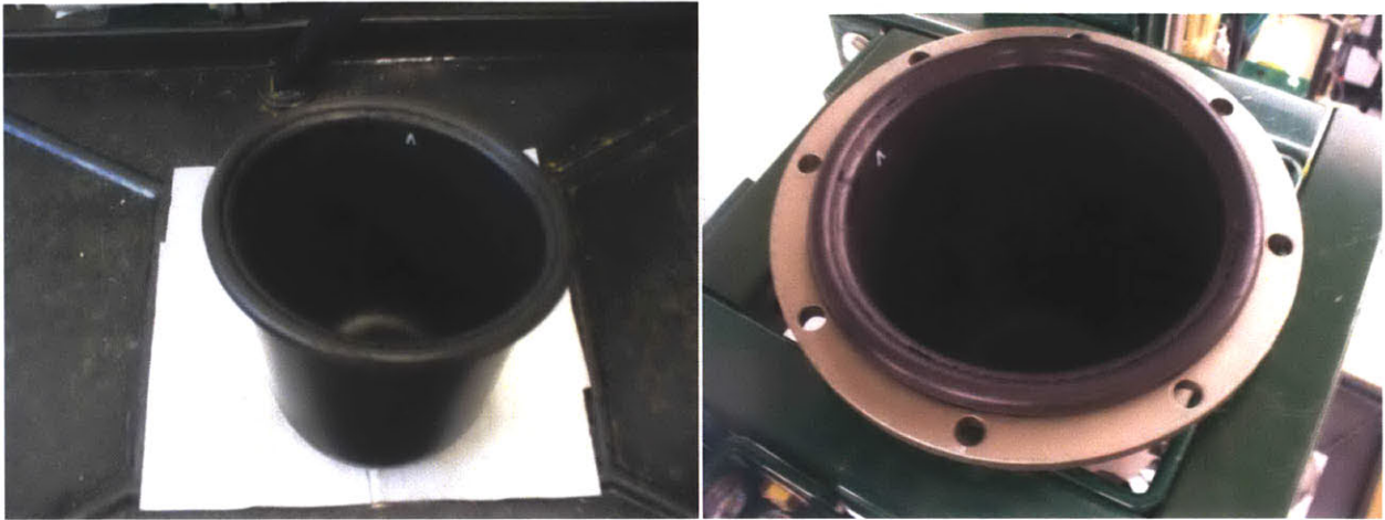
Figure 6-24: Photo of Accumulator Bladder
