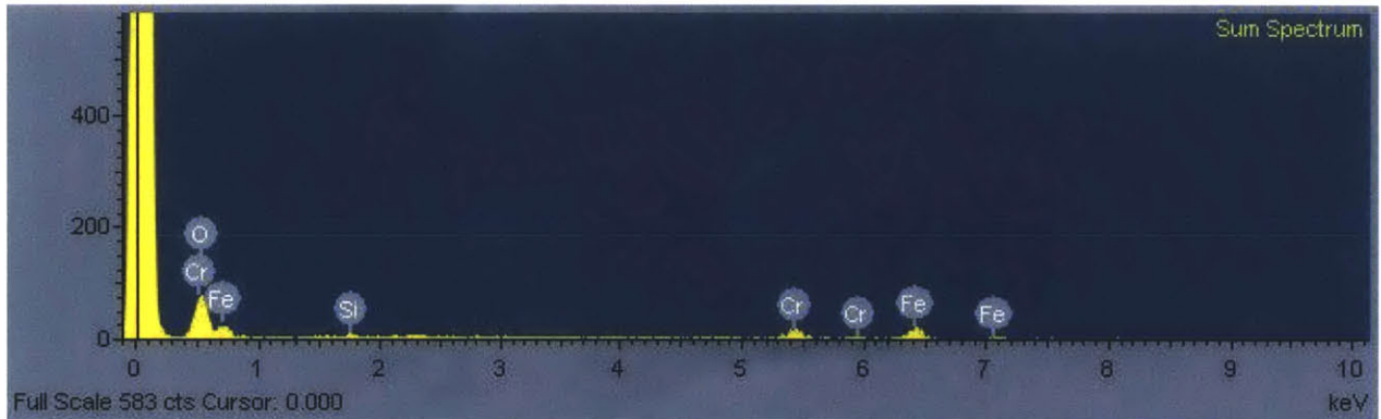
Figure 8-29: EDS of Oxidized SS316L Heater with Sandblast Preparation – DI water - below CHF location
