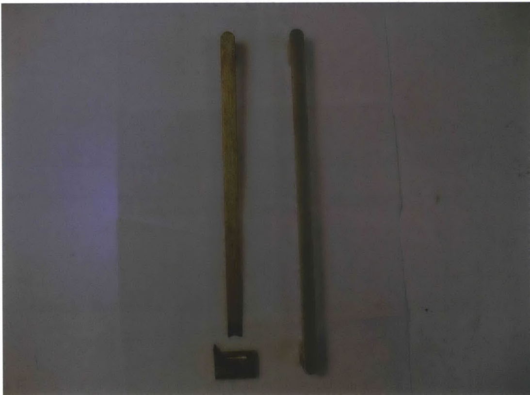
Figure 11-9: Photo of SA508 Heaters: CHF Test (left) and Plain (right)
