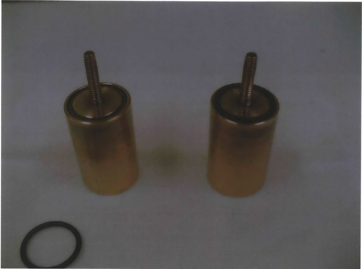
Figure 6-19: Photo of Copper Stud with O-ring
