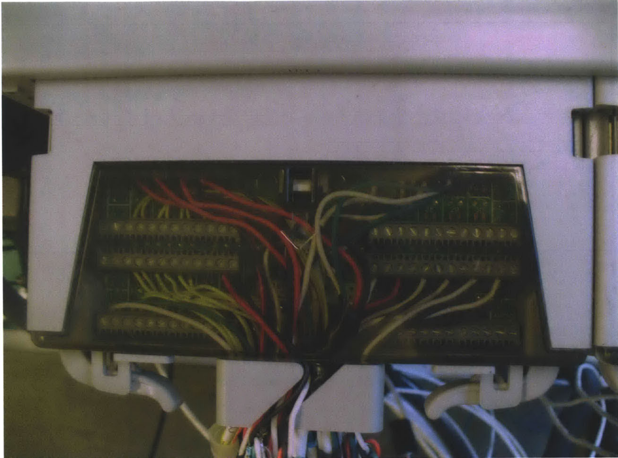
Figure 6-55: Photo of Agilent 34921T Data Card
