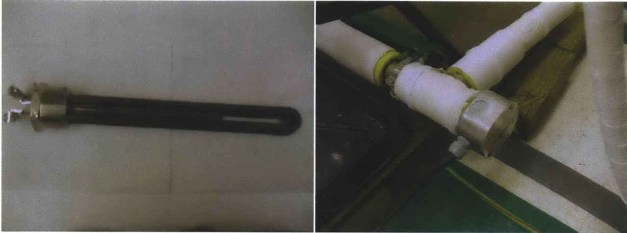
Figure 6-13: Immersion Pre-heater on Test Loop
