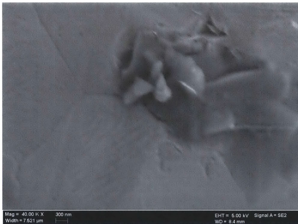
Figure 8-1: SEM of SS316L Unused Heater - Sandblast Preparation - Various Magnification [40,000X]
