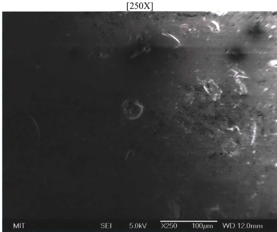
Figure 8-10: SEM of SA-508 - Used in Water - Sandblast Preparation – before CHF location – Various Magnifications
