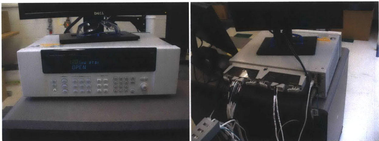
Figure 6-53: Photo of Agilent 34980A DAQ
