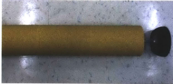
Figure 5-13. Photo of the canister with attached 60 grit sandpaper and drag inducing plug.
