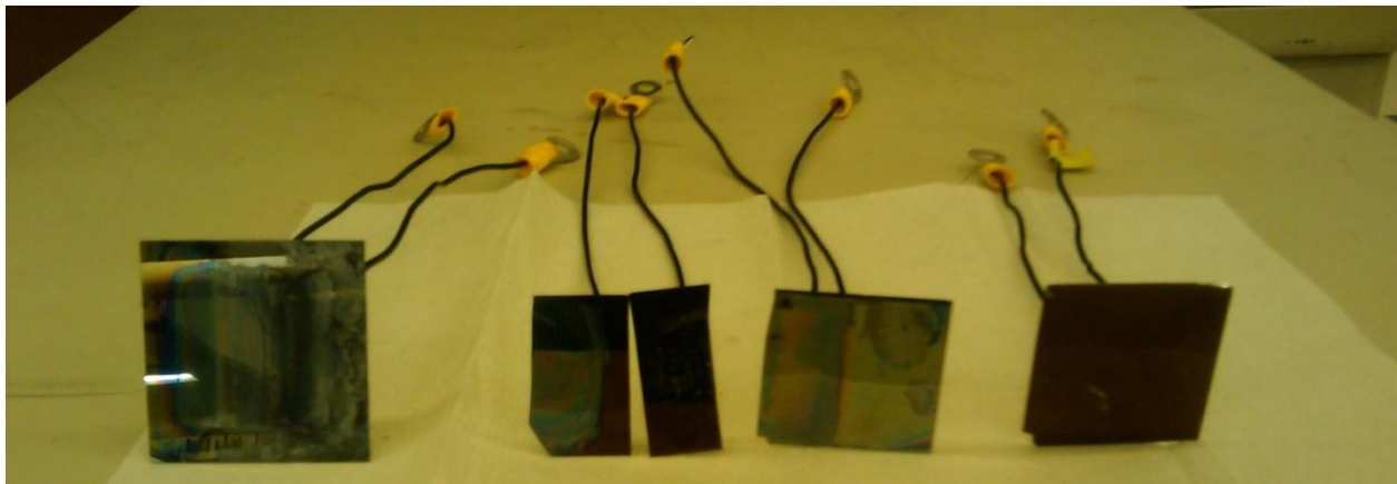
Figure 4-17: Silicon Heaters coated with dielectric coatings. From Left to right, positive electrode is on the left for each heater. 1) Uncoated heater after boiling, large amount of discoloration and deposition 2) Si 3 N 4 heater after test. Some dissolution of the coating on the positive electrode and some aluminum deposition on negative electrode 3) HSQ heater after test slight discoloration on positive electrode, no visible deposition. 4) Clean untested Si 3 N 4 heater. The Si 3 N 4 coating causes the brown discoloration. None of the coatings affected the quality of the IR images.
