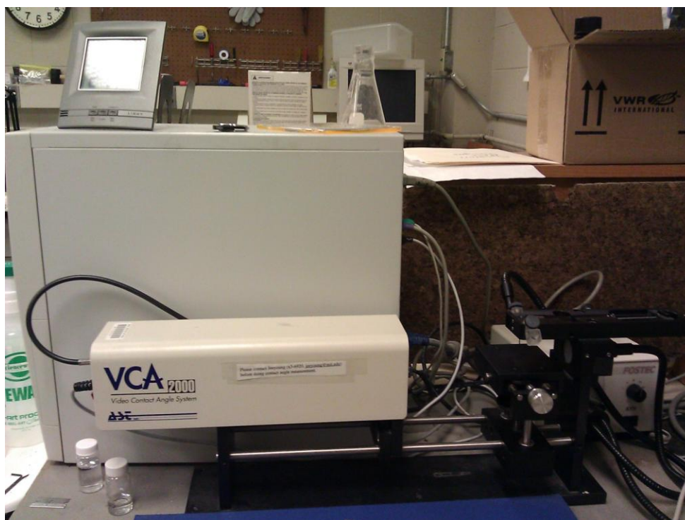
Figure 5-22: AST Products INC VCA 2000 Video Contact Angle System used for contact angle measurements.
