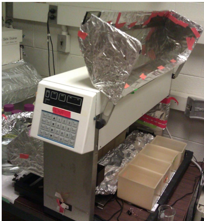
Figure 5-1: Zeiss HMS Programmable Slide Stainer "Wilma". This particular dipper has been modified with large 1L baths positioned on top of stir plates.
