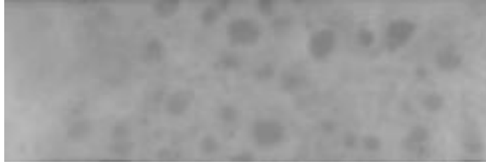
Figure 4-13: 368kW/m 2 heat flux for silicon heater. There is not as good of temperature difference between bubble departures and the rest of the fluid compared to an ITO heater due to measuring the temperature of the water and the relatively low resistivity of the wafer (which reduces transparency). Also, there is a loss of the central hot spot as the center of the bubble dries.
