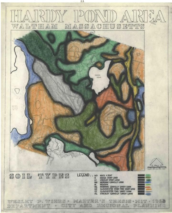
Many of the upper soils are similar, varying only in their porosity and in the amount of ledge or boulder they contain. Few soils, in fact, in the Area are free of coarse materials. Drainage is good but often excessive.
