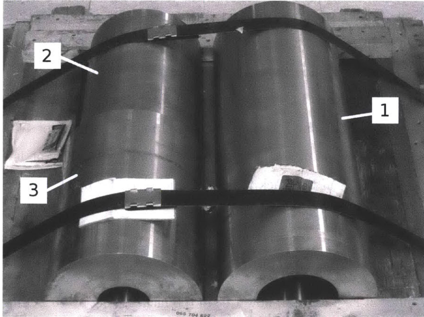
Figure 3-10: Billets of F91 as machined, ready for weld overlaying. The long billet on the right (#1) has been drilled to a 12.7 cm (5") ID to become coolant piping. The billet at the back right (#2) has been lathe-turned down to a 22.9 cm (9") OD to become fuel cladding. The third billet (#3) is to become bare F91 fuel cladding for another project.
