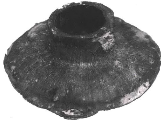
(b) Back end of the OD-clad extrusion billet. The axial grooves present throughout the outer surface of the billet are the beginnings of heat tearing. This is because the cladding (visible as a reddish ring in the cross section) was on the outside, and it clearly was deformed far more in being forced through the mandrel and die during extrusion.
