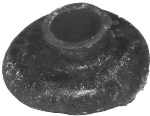
(a) Back end of the ID-clad extrusion billet. Note the regular surface finish, indicating that no heat tearing took place. This is because the cladding (visible as a reddish ring in the cross section) underwent much less deformation being on the ID.
