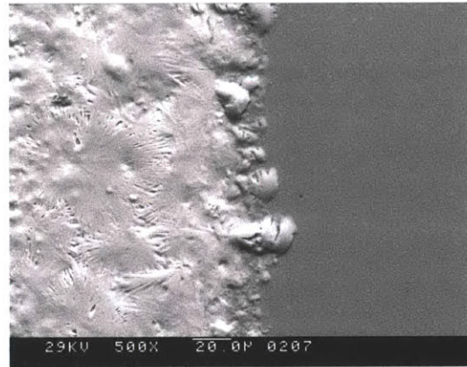
(d) OD-clad FGC exposed to oxidizing LBE far from the interface on the F91 side, 500 \times . LBE has penetrated 20 \mu\text{m} into alloy F91.
