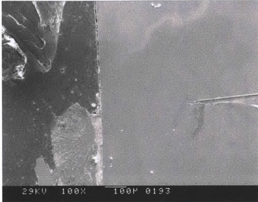
(a) OD-clad FGC exposed to reducing LBE at the bimetal interface, 100 \times . Ferritic grains of Fe-12Cr-2Si are visible on the upper right of the figure. Their termination near the scratch on the right marks the interface.
