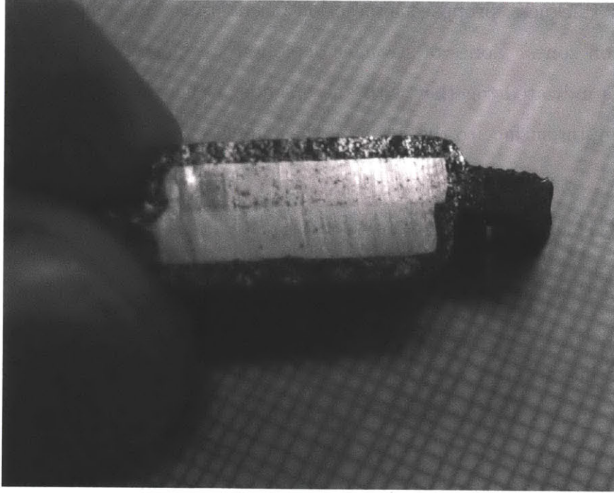
Figure 4-27: Optical macrograph of a diffusion couple as-received from Bodycote, Inc. The carbon steel jacket can be seen surrounding the two metal coupons that make up the diffusion couple. The jacket has rusted due to etching in nital.
