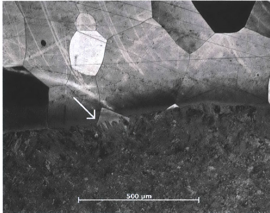
Figure 4-37: Layer interface on the ID-clad weld overlaid billet, 100 \times . Some mixing is present, seen as fingers of martensite poking into a grain of ferrite at the center of the photograph. Overall the interface and mixing layer was very thin.
