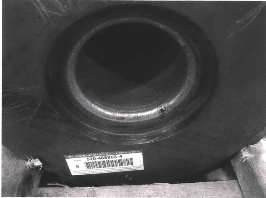
Figure 3-13: Finished ID-clad weld overlaid billet
