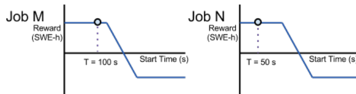
Figure 3-9: Graphs of the current location on the reward functions for two jobs with “by-deadline” SLAs.
