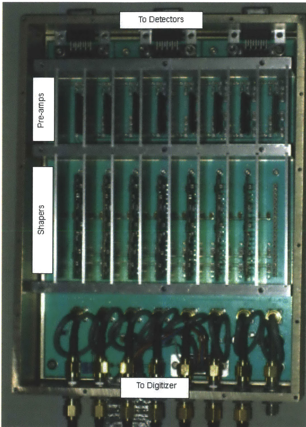
Figure 2-15: The box housing the J-Top electronics
