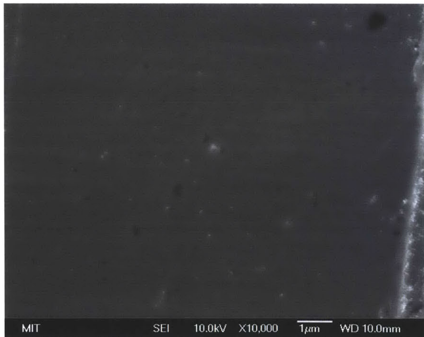
Figure 5-9: Post-test SEM image of heater representative of 1 s transient test
