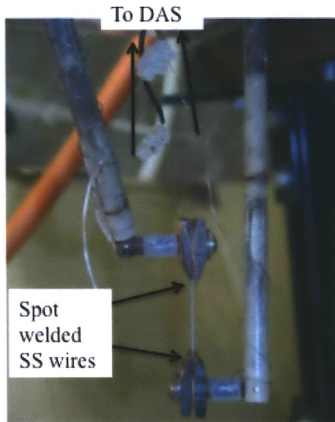
Figure 3-21: Spot-welds across the heated length. The spot-welded wires go to DAS
