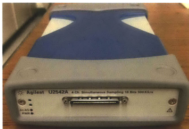
Figure 5-4: Photograph of the U2542A unit used for data acquisition during transient tests
