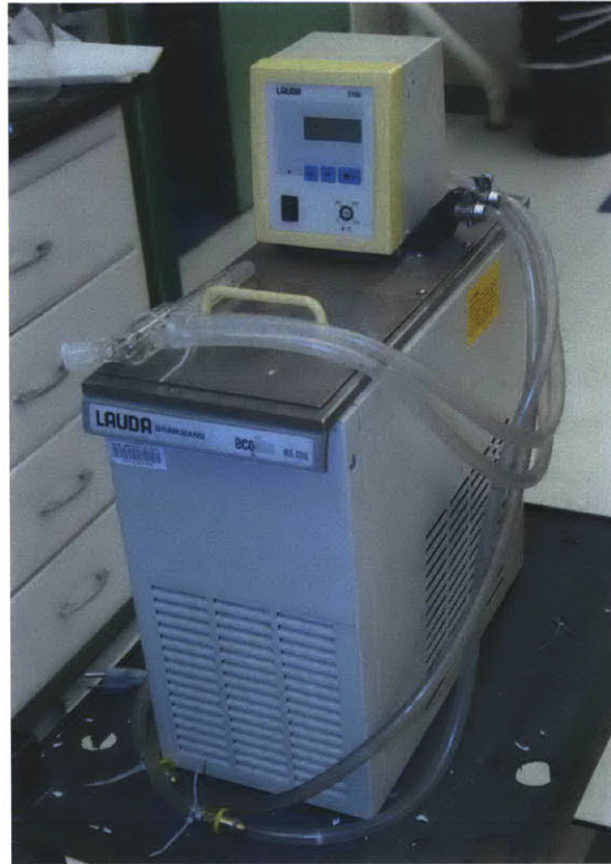
Figure 3-25: Photograph of the chiller used to supply chilled water to the condenser
