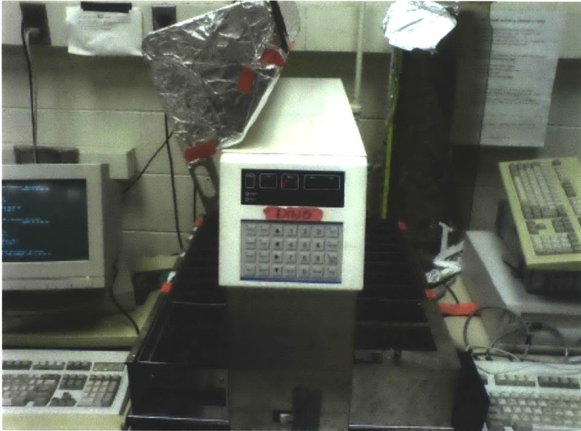
Figure 4-22: Photograph of the Zeiss HMS Programmable Strainer used for coating heater elements with LbL coatings, to change initial surface wettability
