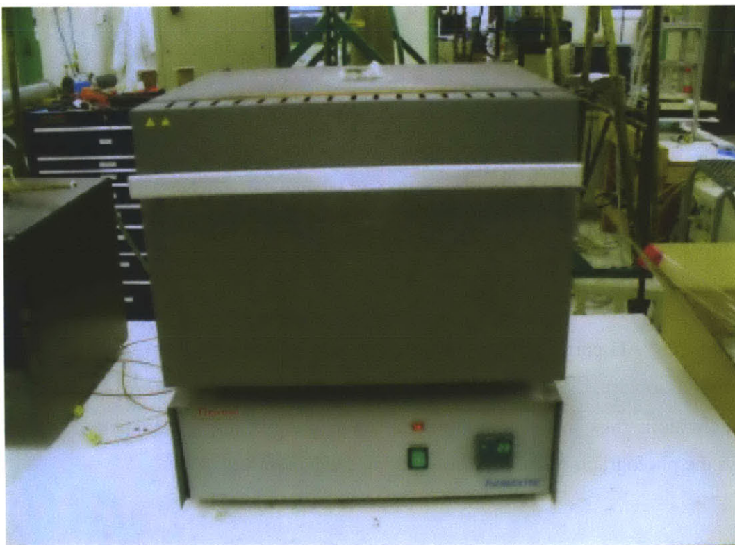
Figure 4-24: Photograph of the furnace used for calcination
