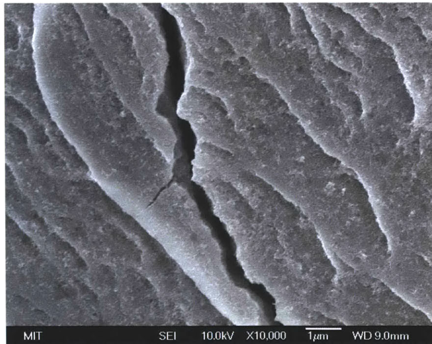
Figure 4-32: Post-test SEM image of heater tested for LbLSB_NF, showing an additional layer of ZnO nanoparticles
