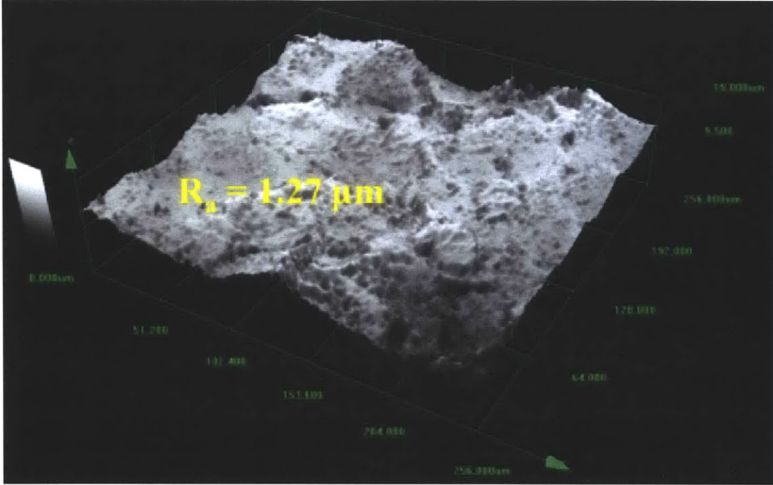
Figure 4-5: Confocal scan of an unused sandblasted heater ( R_a = 1.27 \mu\text{m} )
