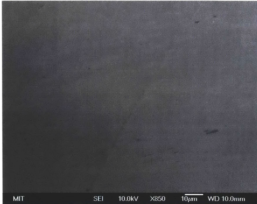
Figure 4-8: SEM image of an unused smooth heater
