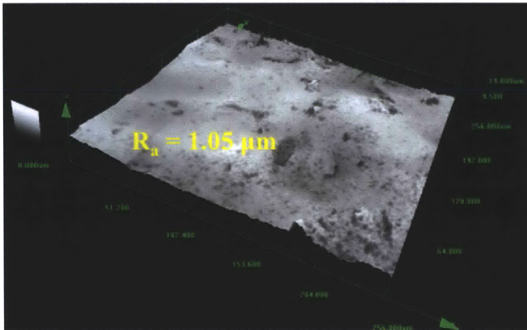
Figure 4-35: Confocal scan of an LbLSB_DIW heater ( R_a = 1.05 \mu\text{m} )
