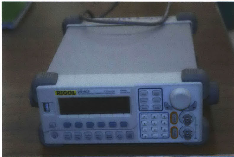
Figure 5-3: Photograph of the function generator to program the power supply for providing desired current outputs
