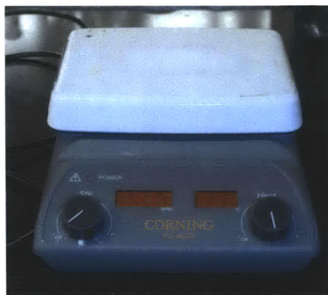
Figure 3-23: Photograph of the hot plate used to maintain the contents of the test-bath at 100 °C
