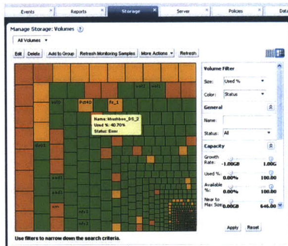
Figure 3. An example of a treemap, a visual representation of how storage is divided. A user can hover over a block and see the status of the storage. They can also click and drill into it to view more details.
