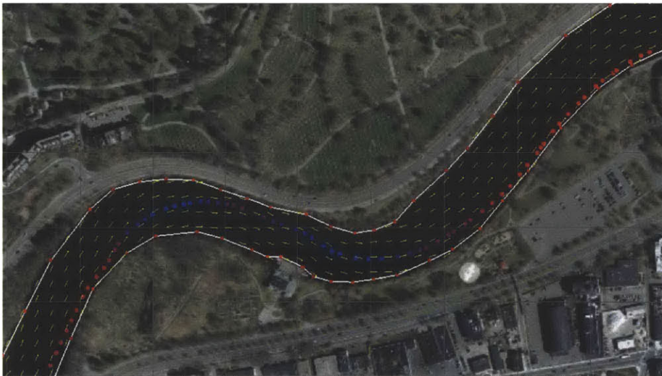
Figure 2-2: Track of simulated passive drifter. The color of the dots represents depth. Deep blue represents deeper water, while bright red represents shallower water. Yellow arrows show the direction of local water currents.
