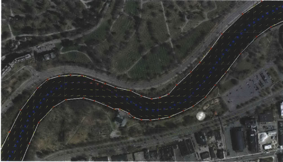
Figure 3-5: Simulation of ARE in thalweg-following behavior. Yellow arrows show local water currents. Colored dots represent places where vehicle took measurements. Depth of measurements is on a false color scale. Deep blue indicates deeper water while bright red indicates shallower water.
