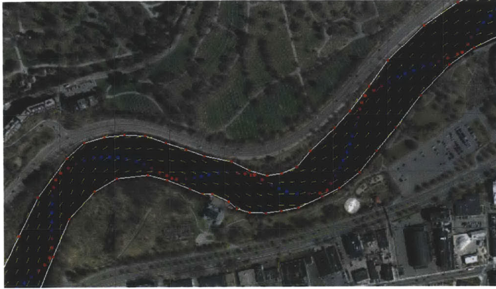
Figure 3-2: Simulated ARE exploring riverine environment. The yellow arrows show local water currents. The colored dots represent places where the vehicle took measurements. The depth of the measurements is on a false color scale. Deep blue indicates deeper water while bright red indicates shallower water.
