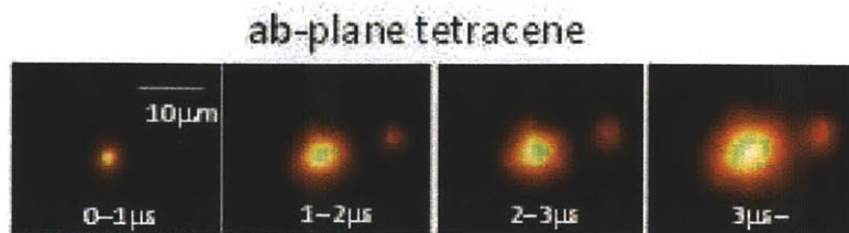
Figure 3-6: Delayed Fluorescence in AB plane axis of Tetracene crystal [13]
