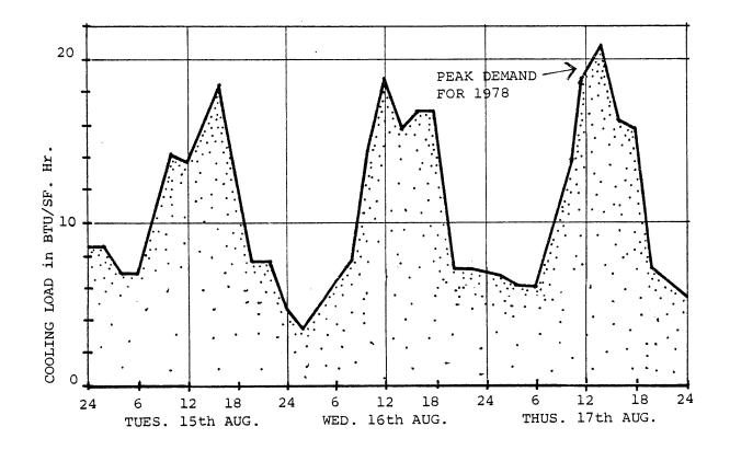
FIGURE 40 Actual Cooling Loads from Monitored Building, August 1978. (courtesy C. Benton)
