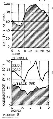
DAILY LOAD CURVE is a graphical representation of electrical demsnd vs. time over a 24 hour cycle. This demand may be the needs of a customer or the load placed on a utility system. The highest point on the graph represents the time and magnitude of the day's peak load. The illustration represents a summer peak day for Boston Edison.<sup>14</sup>
