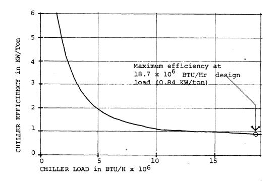
FIGURE 39 Chiller Efficiency vs. Load in Monitored Building (courtesy C. Benton)
