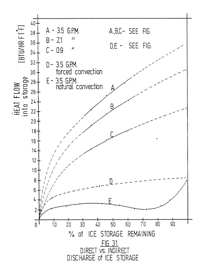
able to absorb any anticipated cooling load. This is only true if the tank water being pumped is able to enter the space between the pipe wall and the ice cylinder throughout the course of the discharge period. The piping would have to be designed to facilitate this.
