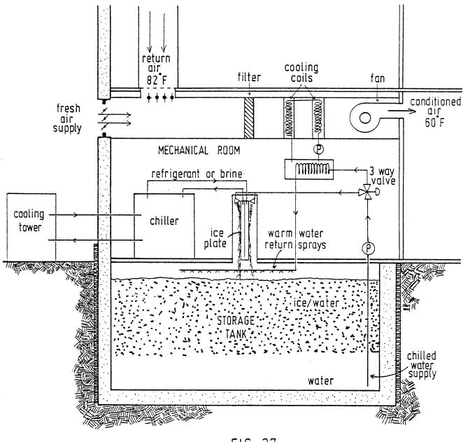
FIG 37 ICE STORAGE USING A FROSTLESS ICE PLATE
