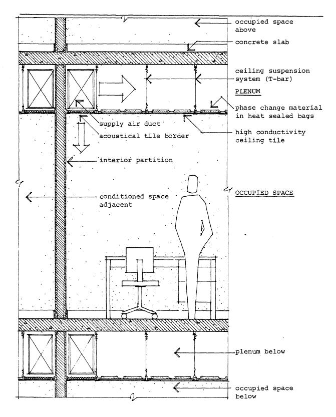
FIGURE 11 Vertical Section Through Interior Zone Space Showing System Components. (courtesy C. Benton)
