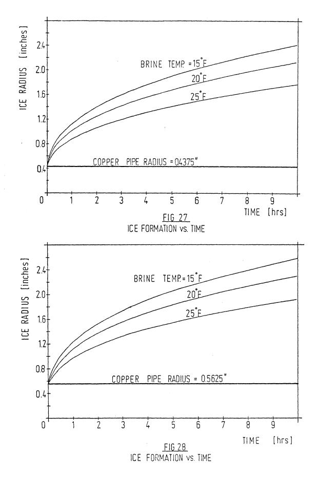
The plastic pipe considerably retards the formation of ice due to its poor thermal conductivity for 5/8" pipe at 20°F. The copper pipe will form 77% more ice in 10 hours than the plastic pipe which means 77% more plastic pipe is needed to make the same amount of ice per unit of time. By knowing the ice radius, the proper pipe spacing is determined (double the radius). Figures 26, 27, 28 show ice radii for other pipe sizes and brine temperatures.
