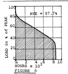
LOAD DURATION CURVE portrays the same information contained in the previous load curves except for the timing of demand. Demand values are plotted in descending order with 24 hour values for a yearly curve. This graph is normally constructed for utility systems and is useful for visualizing the character of peakload vs. baseload. This curve represents Boston Edison data in 1978.<sup>16</sup>
