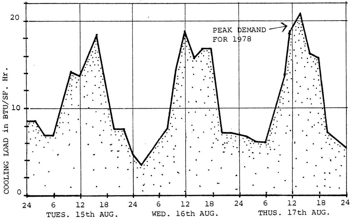
FIGURE 40 Actual Cooling Loads from Monitored Building, August 1978.
