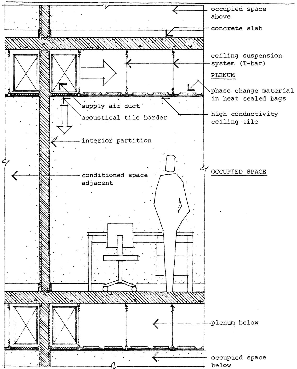
**FIGURE 11** Vertical Section Through Interior Zone Space Showing System Components.
