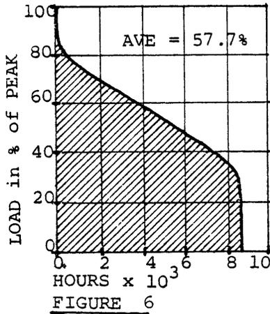
LOAD DURATION CURVE portrays the same information contained in the previous load curves except for the timing of demand. Demand values are plotted in descending order with 24 hour values for a yearly curve. This graph is normally constructed for utility systems and is useful for visualizing the character of peakload vs. baseload. This curve represents Boston Edison data in 1978.<sup>16</sup>
