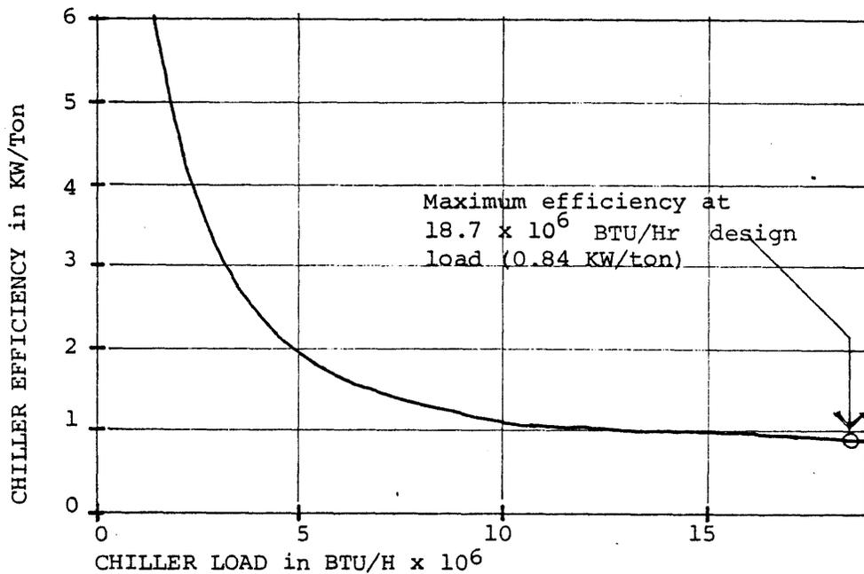
FIGURE 39 Chiller Efficiency vs. Load in Monitored Building
