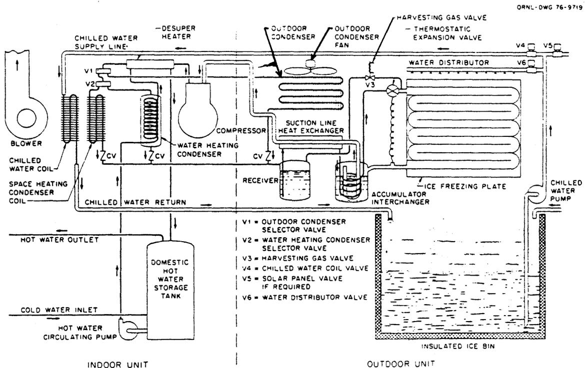
Fig.14. Schematic drawing of the ACES ice-maker heat pump
