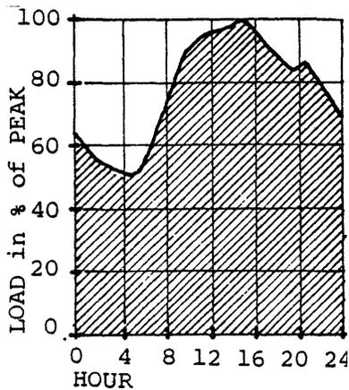
DAILY LOAD CURVE is a graphical representation of electrical demand vs. time over a 24 hour cycle. This demand may be the needs of a customer or the load placed on a utility system. The highest point on the graph represents the time and magnitude of the day's peak load. The illustration represents a summer peak day for Boston Edison.<sup>14</sup>
