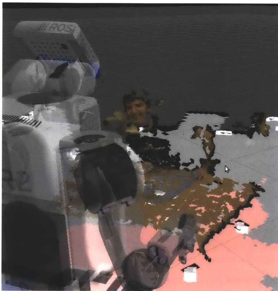
Figure 3-1: The RP2 depth sensor has high accuracy and can perceive different types of objects and subjects, even humans. In this rendering, the author is perceived as a point cloud, next to a table in front of the robot.
