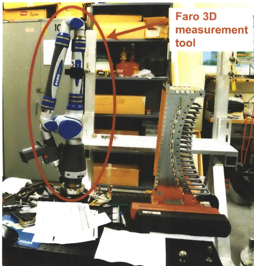
Figure 6-4: This is an image of one of two Faro coordinate measuring machines (CMMs) used to check alignment and manufacturing specifications.
