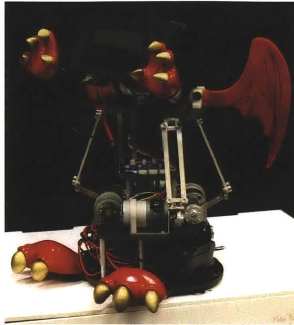
Figure 3-32: DragonBot V4 prototype with 3D printed aesthetics
