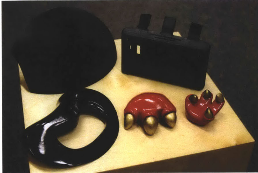
Figure 3-27: 3D printed parts for DragonBot (clockwise from upper left): cranium (FDM), head (FDM), hand (MJM), foot (MJM), faceplate (MJM)
