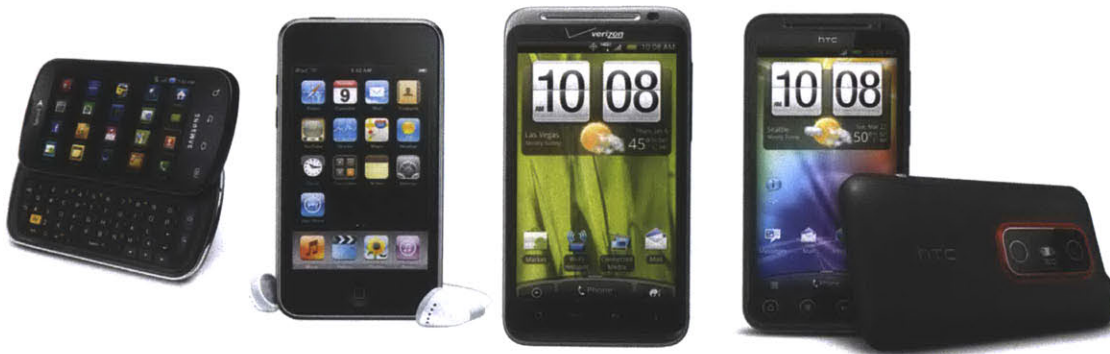
Figure 3-21: The mobile devices used for the DragonBot prototypes (from left to right): Samsung Galaxy Epic (V1), iPod touch (V2), HTC Thunderbolt (v3), HTC Evo 3D (V4 and V5)
