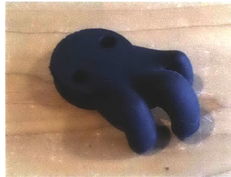
Figure 3-31: Foot prototype, urethane-iron hybrid material
